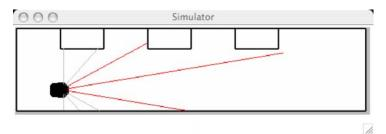
Part of the robot model is an error model for the sonar readings. Our error model for sonar readings will have a similar structure to the error model for observing colors in the hallway: we determine the sonar observation we would expect to see in each state, if our observations were perfect, and then use that as the basis for constructing a distribution over possible observations.
